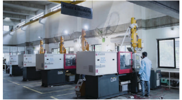
Plastic Enclosure Manufacturing In-house Injection Moulding
